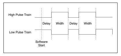
Figure 4-3. High and Low Pulse Trains
